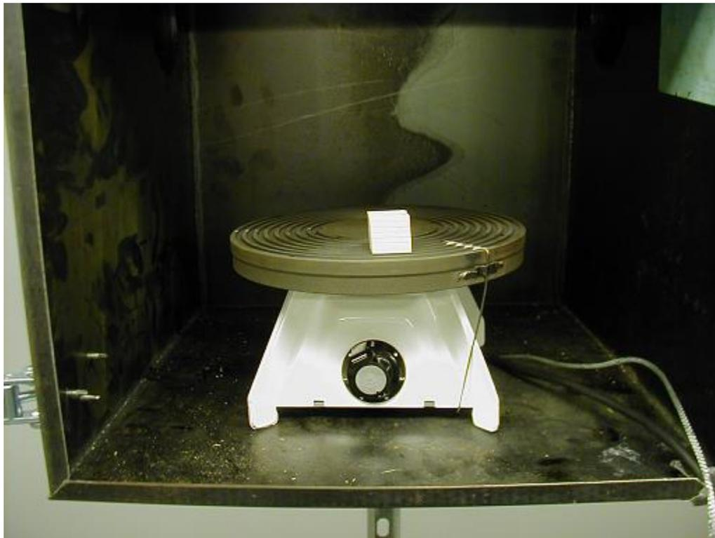
Photo of inside of smoke generation chamber
